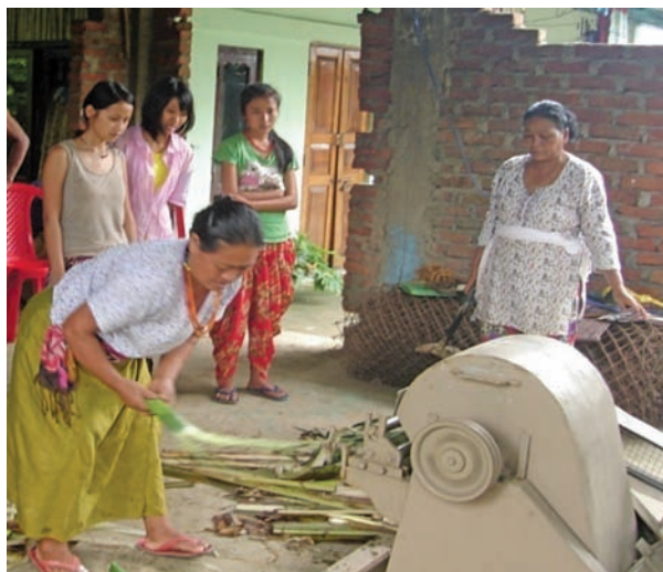
Extraction of Banana Fibre
