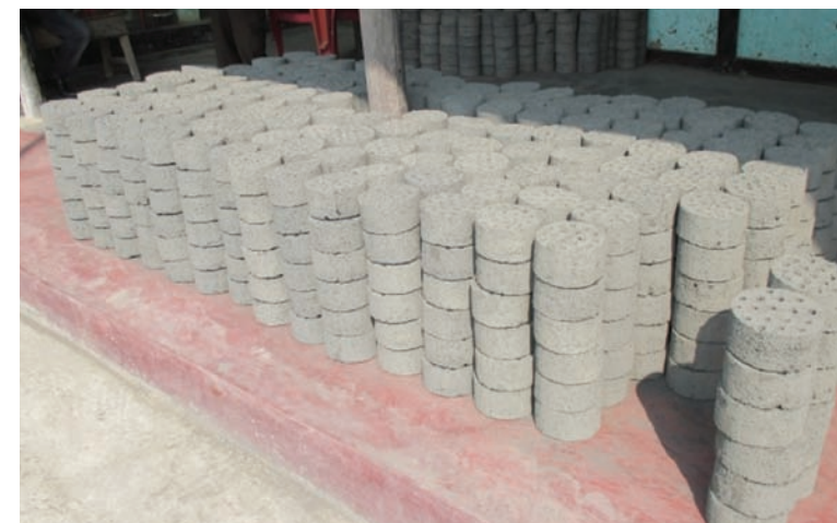
Drying of beehive briquette
